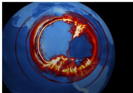
*Snapshot of a seismic wavefield modelled with our in-house methods. Simulations for 1 Million New-Zealand earthquake models.*
