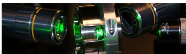
The aim of this project is to develop a new experimental capability, using rapid transient grating spectroscopy (TGS) measurements to probe the elastic, i.e. seismic, properties of Earth materials in a Diamond Anvil Cell (DAC). TGS has the potential to allow measurements up to 4 orders
