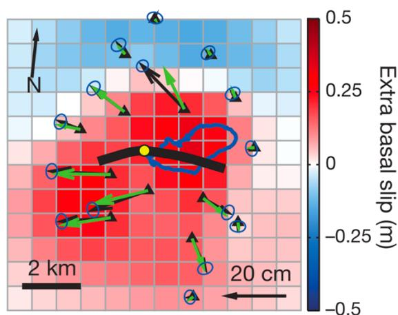
GPS displacements (green arrows from black triangles) and Network Inversion Filter-calculated extra basal slip (colorbar) during the rapid drainage of a single supraglacial lake [Stevens *et al.*, 2015]. Moulin location, last known lake shoreline, and hydro-fracture surface trace are shown as a yellow circle, blue line, and black line, respectively. A project goal is to determine how stress is transmitted between neighbouring lake basins during the drainage of one or more lakes.
