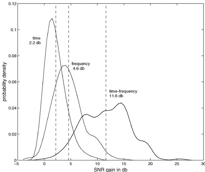
Fig. 11. Histogram of relative method gains in decibels of the three first-order schemes over the zeroth-order scheme, i.e.,  $\text{SNR}_{tf} - \text{SNR}_c$ ,  $\text{SNR}_t - \text{SNR}_c$ , and  $\text{SNR}_f - \text{SNR}_c$ .
