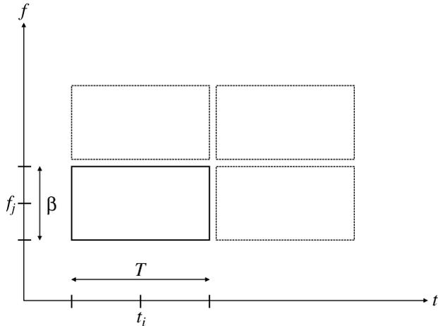
Fig. 2. Dividing up the global time-bandwidth resource into blocks of duration  $T$  and bandwidth  $B$ ; channel model parameters need to be estimated for every block. If the channel varies both temporally and spectrally, then both kinds of fluctuations should be included in the modeling to maximize the SNR after demodulation and to keep the training overhead low.
