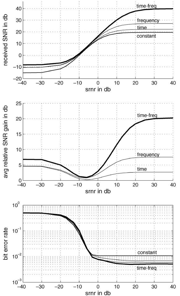
Fig. 12. Estimation results for wireless simulations, as a function of the signal-to-added-noise level (snr) at the receiver. The channels had temporal and spectral fluctuations of the magnitudes expected for cellular communications in cars (refer to the text for parameters and definitions). (Top) Average received SNR for all four estimation methods. (Middle) Average SNR gains of the three first-order methods over the constant-only method. (Bottom) BERs for a binary constellation.
