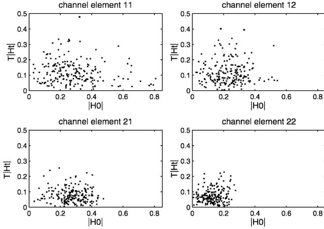
Fig. 8. Estimated magnitudes of first-order temporal variation  $T|H^t|$  versus constant channel attenuation  $|H^c|$  for the 200 acoustic  $2 \times 2$  MIMO channels measured in the acoustic experiment.
