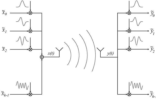
Fig. 5. Communication scheme for the single-antenna case.  $K$  symbols are modulated by  $K$  Slepian pulse-shaping functions, transmitted over the temporally and spectrally varying channel, and demodulated by a bank of  $K$  matched filters.
