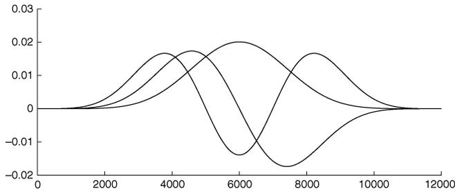
Fig. 3. First three discrete prolate spheroidal sequences, also called Slepian sequences ( $T = 2.4$  s,  $B = 5$  Hz,  $K = 11$ ,  $n = 12000$ ).
