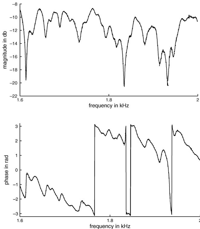
Fig. 6. Magnitude and phase of an acoustic channel transfer function, as measured in the quiet and empty Bell Labs cafeteria. Fades are spaced by about 20 Hz.
