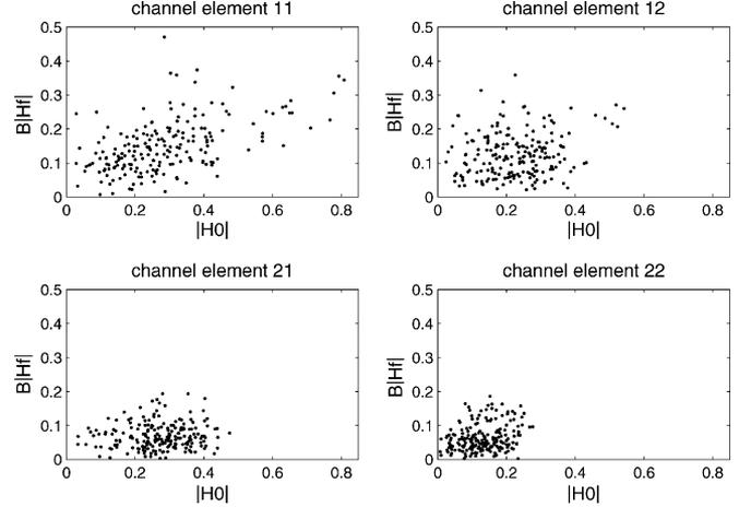
Fig. 9. Estimated magnitudes of first-order spectral variation  $B|H^f|$  versus constant channel attenuation  $|H^c|$  for the 200 acoustic  $2 \times 2$  MIMO channels measured in our experiment.
