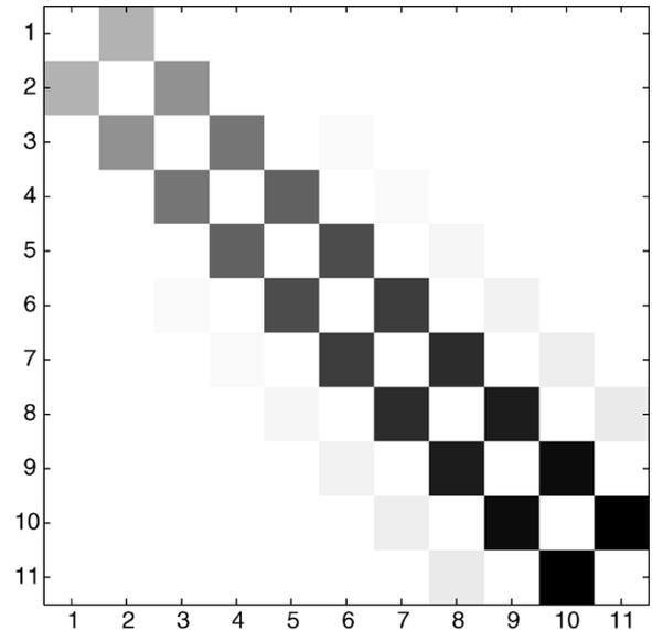
Fig. 4. Magnitude of elements of the  $11 \times 11$  time operator  $\mathbf{T}$  in the Slepian basis. A plot of the frequency operator  $\mathbf{F}$  looks almost identical. Both matrices are practically bidiagonal, but the time operator is real and symmetric, whereas the frequency operator is purely imaginary and skew-symmetric. This difference allows us to distinguish between time variation and frequency variation in the channel.
