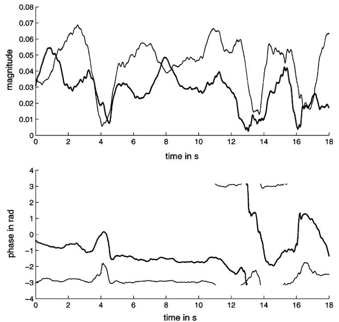
Fig. 7. Temporally varying amplitudes of two acoustic tones at 1500 and 1520 Hz, measured in the Bell Labs cafeteria during lunch time. The time scale of amplitude fluctuations is on the order of 1 sec; amplitudes vary over roughly one order of magnitude.
